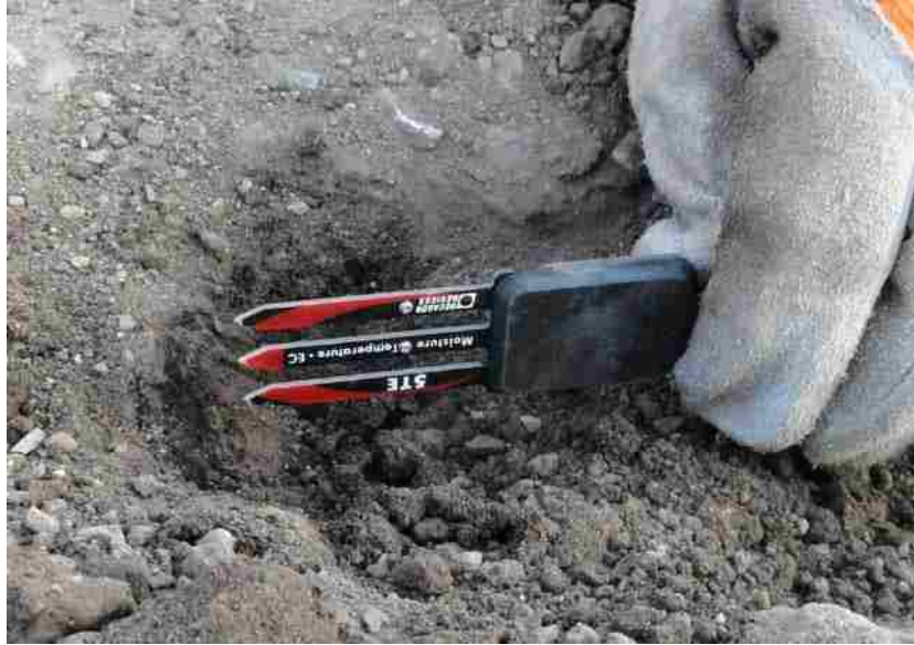
Figure 3-4: Soil moisture, temperature, and electrical conductivity sensor.
