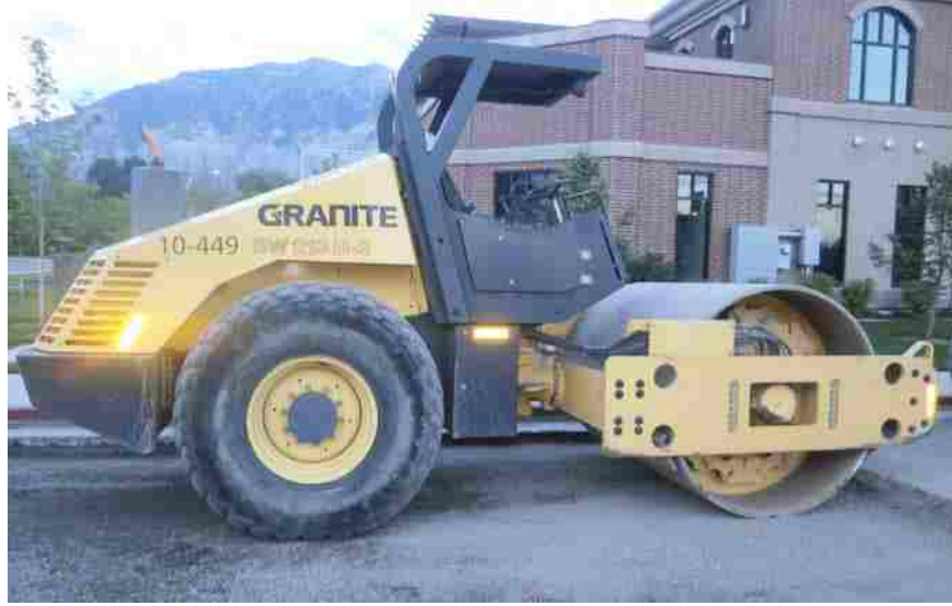
Figure 3-6: Vibratory roller for compaction of base layer at Orem site.
